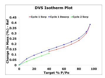
In the image below, the recorded sorption/desorption profile shows hysteresis in the range 40-60% RH. Hysteresis usually suggests a phase change with formation of a hydrate by absorption of water molecules in the structure:
