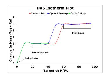
In the picture below, the typical sorption/desorption profile for a channel hydrate is observed: hydrated and dehydrated structures are isomorphic (i.e. no hysteresis during hydration/dehydration). Hence, the water sorption and desorption appear as overlapping reversible cycles.
